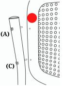
Please locate top of backrest and position the backrest facing up. You will see color codes on screw (A) which will match the color code on the back of the frame to verify the backrest is positioned correctly.
